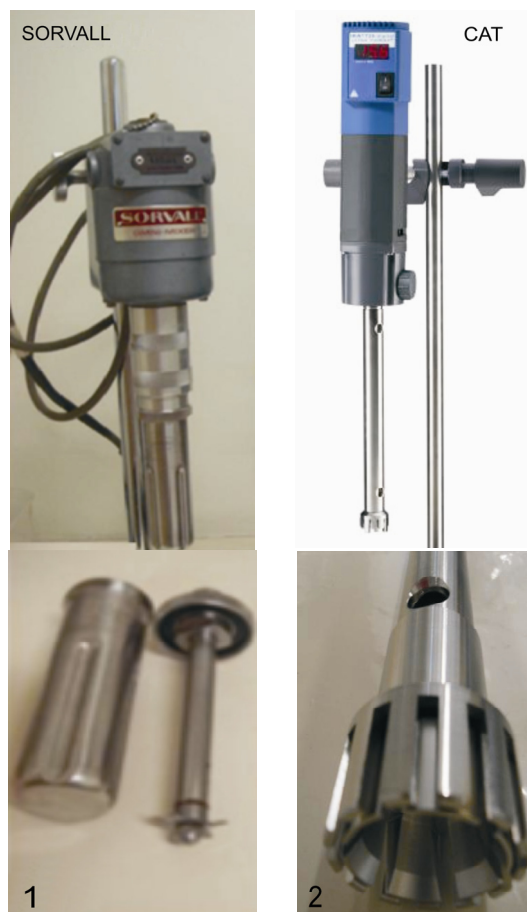
Figure 4: The two types of homogenisers used in the present study. (1) Sorvall Omni Mixer, which has a helical axis inside a reservoir; (2) CAT, which has two overlapping axes, a fixed and a mobile one.
