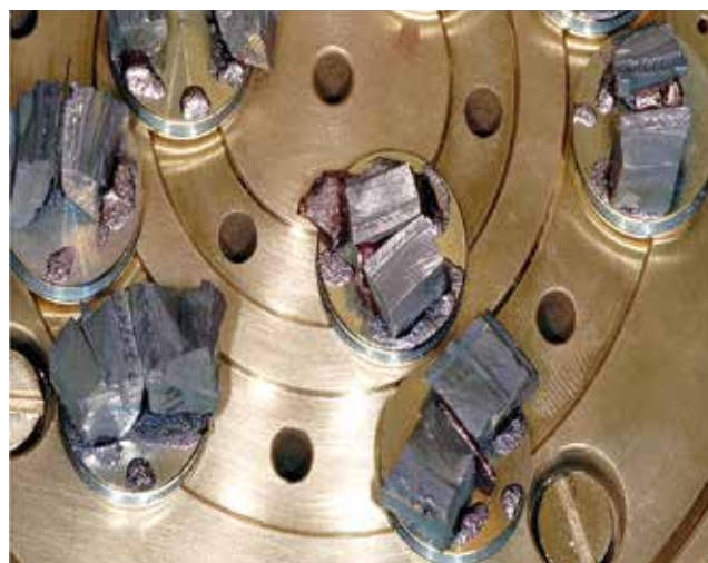
Figure 5 - Metallized specimens placed on stubs.
