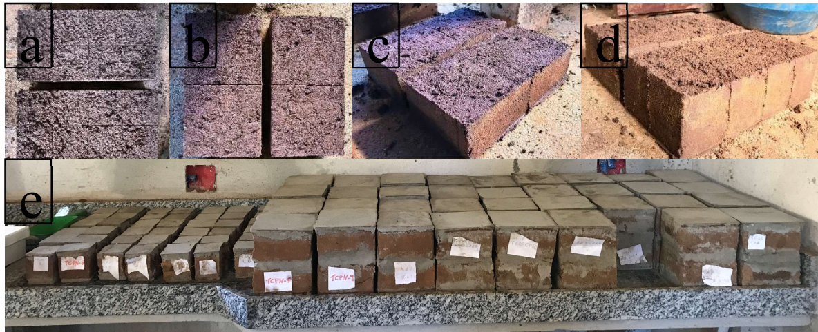
FIGURE 5. Preparation of adobes for the compressive test according to NTE E 080 and Brazilian standard. Superior view of the adobes cut by the Brazilian standard (a), superior view of the adobes cut by NTE.E-080 (b), lateral view of the adobes cut by NTE.E-080 (c), lateral view of the adobes cut by the Brazilian standard (d), adobes capped and ready for testing (e).
