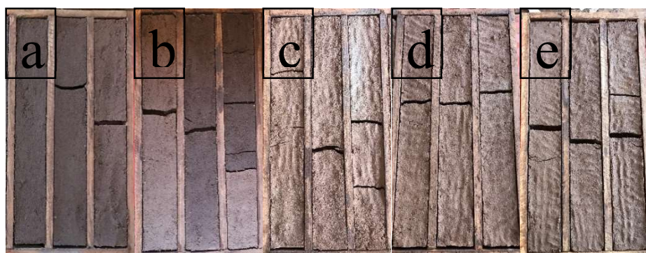
FIGURE 10. Linear shrinkage of adobes after 7 days of drying. Control (A), S1 (B), S3 (C), S5 (D) and S7 (E).
