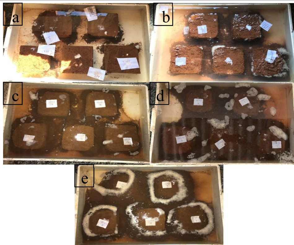
FIGURE 9. Adobes after 6 hours of submersion in water. Control (a), S1 (b), S3 (c), S5 (d) and S7 (e).
