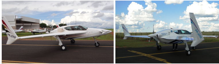
Figure 1. Typical canard-type aircraft. (Courtesy of FABE Ltd.).
