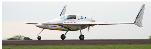
Figure 23. Canard aircraft with semicircular scoop (Courtesy FABE Ltd.).
