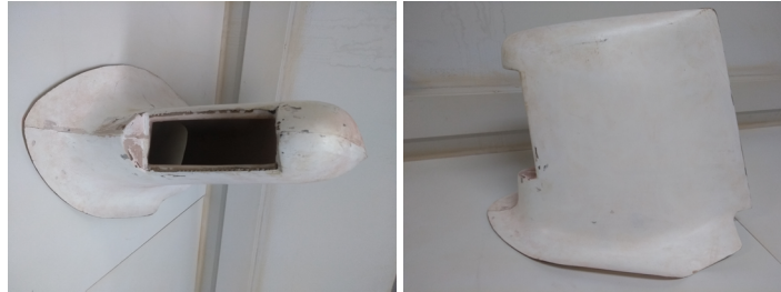
Figure 10. Standard air intake (Courtesy of FABE Ltd.).
