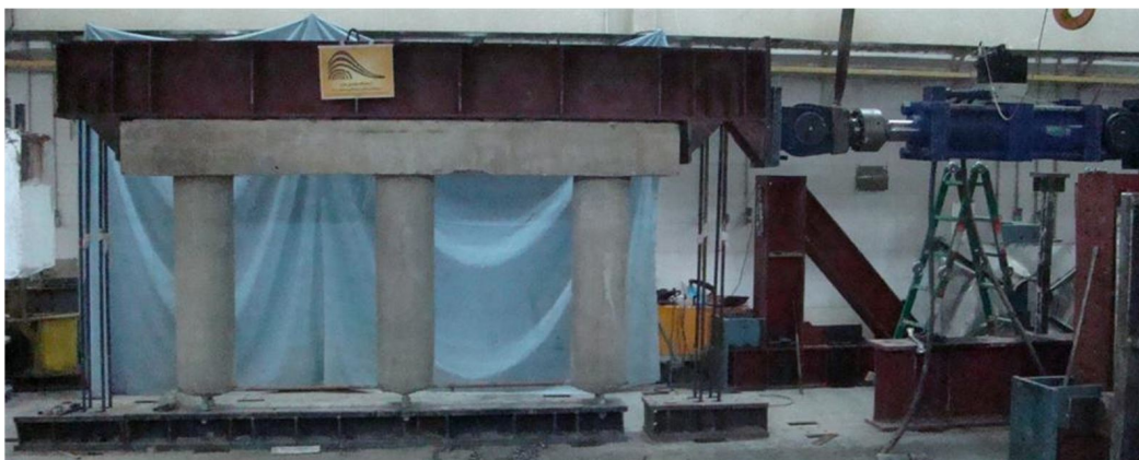
Figure 4: Specimen designed based on 90s code (specimen A).
