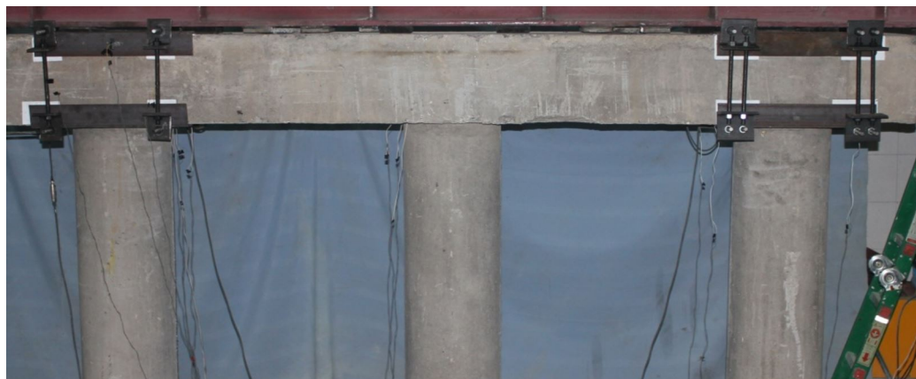
Figure 5: Retrofitted specimen with one side external pre-stressing (specimen B).
