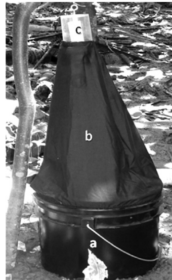
Fig. 2: emergence trap. a: black plastic cylinder: 26.5 cm high and 30 cm diameter; b: black cloth in form of truncated cone 46 cm high, which permits teneral insects to move toward the collecting recipient; c: transparent collecting container: 12 cm high, 6 cm diameter with a concentric cylindrical tube: 9 cm high, 3 cm diameter, it was impregnated with castor oil to trap insects.
