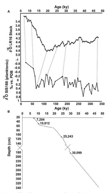
Figure 2. Age model of the core SIS188. (A) Correlation between Lisiecki and Stern (2016) South Atlantic intermediate standard curve and the oxygen isotope data from the marine core SIS188 (presented by Duque-Castaño et al. 2019). (B) Relationship between age and depth in the marine core SIS188. The dots are the depths where radiocarbon dating was performed.
