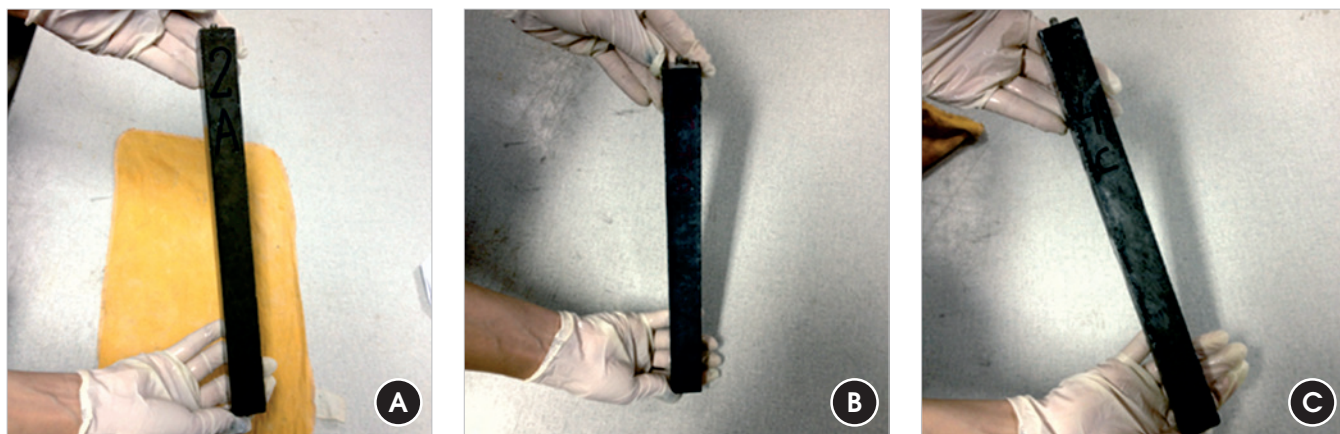
Figure 5 – Prismatic bars used in the expansion evaluation (a) placed in curing room after 327 days – (b) placed in the Ca(OH) 2 solution kept at room temperature after 320 days (c) placed in the Ca(OH) 2 solution kept at 50°C after 313 days
